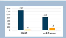
"The high durability and operational efficiency of tungsten carbide coating over traditional hard chrome plating is scientifically evidenced by its ability to withstand higher levels of wear and provide extended operational lifespan"
